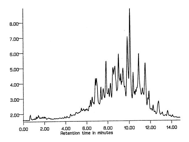
Toxaphene analyzed on an SPB-608 fused-silica open-tubular column. The GC operating conditions were as follows: 30 m x 0.53 mm ID SPB-608. Temperature program: 200°C (2 min hold) to 290°C at 6°C/min.
