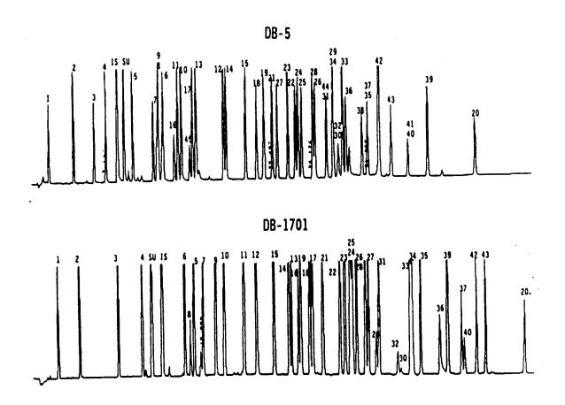
Organochlorine pesticides analyzed on a DB-5/DB-1701 fused-silica open-tubular column pair. The GC operating conditions were as follows:  $30 \text{ m} \times 0.53 \text{ mm}$  ID DB-5 (0.83- $\mu$ m film thickness) and  $30 \text{ m} \times 0.53 \text{ mm}$  ID DB-1701 (1.0- $\mu$ m film thickness) connected to an 8 in. injection tee (Supelco Inc.). Temperature program:  $140^{\circ}\text{C}$  (2 min hold) to  $270^{\circ}\text{C}$  (1 min hold) at  $2.8^{\circ}\text{C/min}$ .
