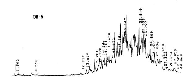
Strobane analyzed on a DB-5/DB-1701 fused-silica open-tubular column pair. The GC operating conditions were as follows: 30 m x 0.53 mm ID DB-5 (1.5- $\mu$ m film thickness) and 30 m x 0.53 mm ID DB-1701 (1.0- $\mu$ m film thickness) connected to a J&W Scientific press-fit Y-shaped inlet splitter. Temperature program: 150°C (0.5 min hold) to 190°C (2 min hold) at 12°C/min then to 275°C (10 min hold) at 4°C/min.
