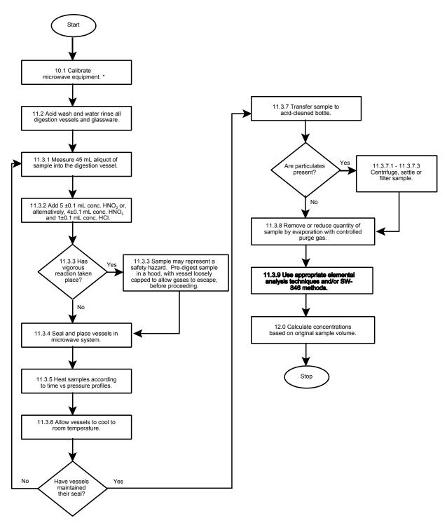
\* Not necessary if using a unit equipped with temperature feedback control.
